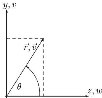
Figure 1: Polar and cartesian coordinate system definitions.
